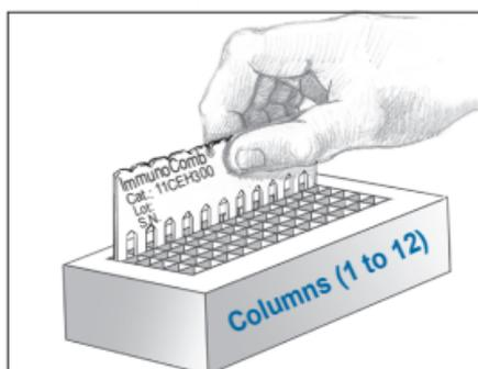
■ Upon completion of the color development in row F, move the Comb back to row E for 2 minutes for color fixation. Take the Comb out and let it dry for 5 minutes before reading the results.
