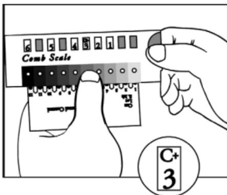
**While holding the ruler,** find the tone of purple-grey on the CombScale that most closely matches the desired **test result spot** (one of the lower spots).
