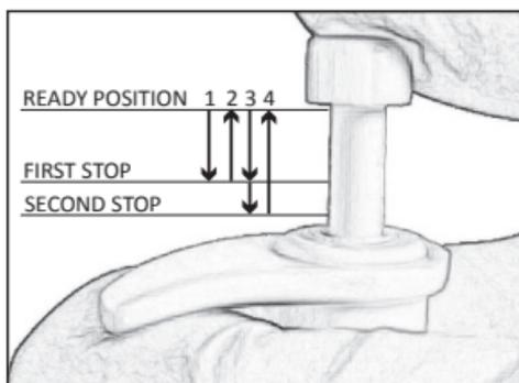
3- Dispense the sample into a well in row A by gently pressing the operating button to the first stop. After a second, press the operating button to the second stop. This will empty the tip completely. Remove the pipette from the well.
